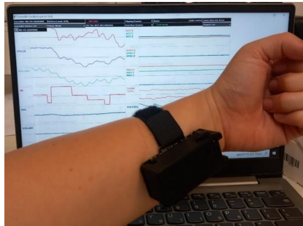
Figure 3 – Emotibit sensor with a case on the wrist and the EmotiBit Oscilloscope software
